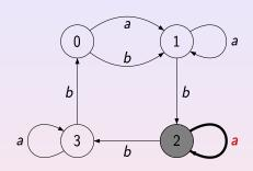
A reset word is w = abbbabba: applying it at any state brings the automaton to the state 1.
