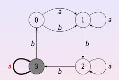
A reset word is w = abbbabbba: applying it at any state brings the automaton to the state 1.
