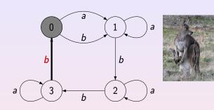
A reset word is w = abbbabbba: applying it at any state brings the automaton to the state 1.
