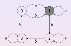
A reset word is w = abbbabba: applying it at any state brings the automaton to the state 1.
