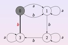
A reset word is *abbbabbba*: applying it at any state brings the automaton to the state 1.
