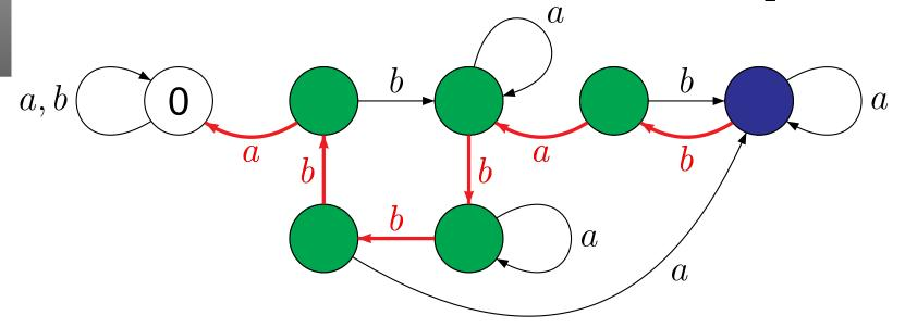
If a synchronizing automata with k states has a unique sink, then it has a reset word of length  $\leq \frac{k(k-1)}{2}$ .
