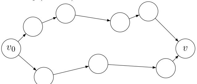
Let  $v \in V_i \cap V_j$  where  $i \neq j$ . This means that in  $\Gamma$  there are two paths from  $v_0$  to v: of length  $\ell \equiv i \pmod{k}$  and of length  $m \equiv j \pmod{k}$ .
