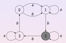
A reset word is *abbbabbba*: applying it at any state brings the automaton to the state 1.
